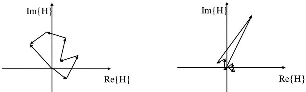
Fig. 2: The complex FRF and its modal components, for one frequency. a) No mode dominates. b) One component is dominating.
