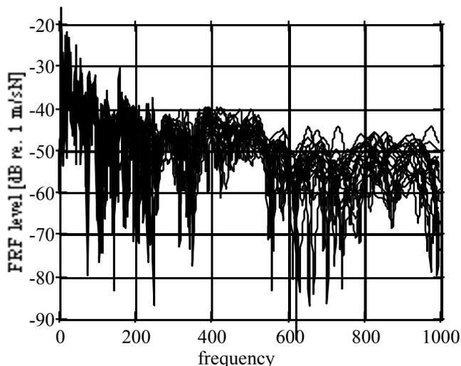
Fig. 5: FRFs for combined random variations of eigen-frequencies and modal damping. Standard deviations: 2% for eigenfrequencies and 20% for the logarithm of damping factor.
