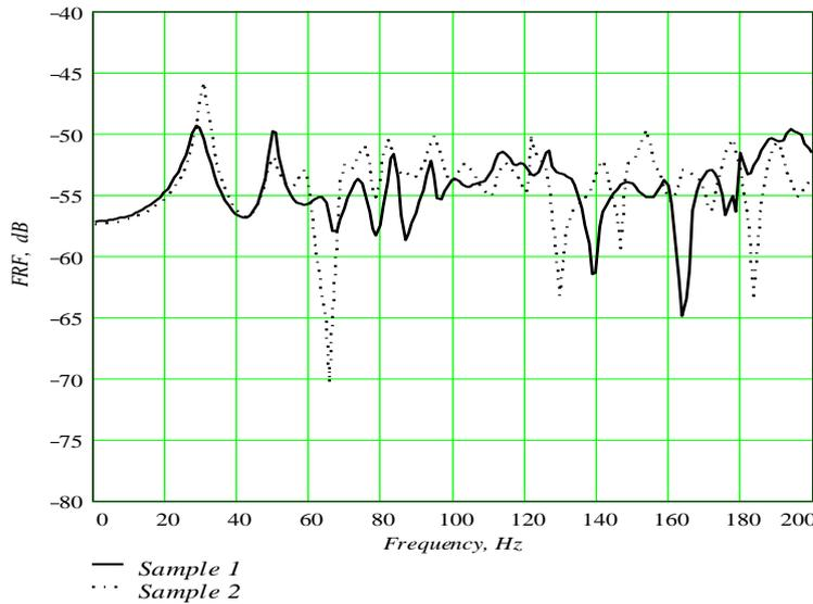
Fig. 3: FRFs for the generic modal expansion model with  $\eta = 5\%$ . Standard deviations: 3% for eigenfrequencies, 30 % for logarithm of the modal damping.
