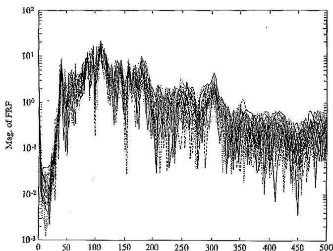
Fig. 1: Magnitudes of the 99 structure-borne FRFs for the RODEOs for the driver microphone [1].
